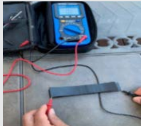
Figure 3. Using ohmmeter to qualify conductive side
