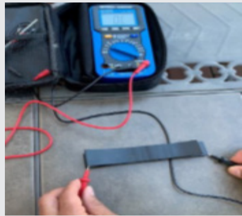
Figure 3. Using ohmmeter to qualify conductive side
