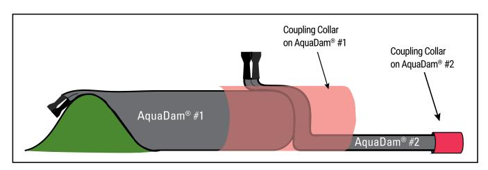
The open end of the AquaDam® #2 should be totally enclosed by the coupling collar. Pull the end of the outer skin of AquaDam® #2 on top of the outer skin of the water filled AquaDam® #1 within the connection collar.
