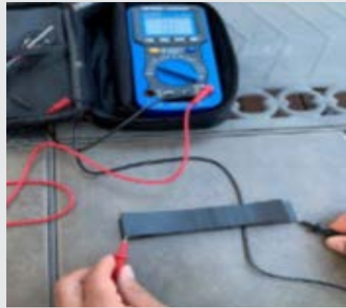
Figure 3. Using ohmmeter to qualify conductive side
