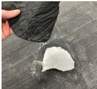
Figure 1: Damaged conductive layer.
